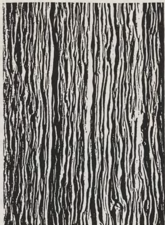
Mold of longitudinal meandering grooves. Run 4 (table 1). Flow from bottom to top. Bed shown is 27 cm wide. ( \bar{U} = 0,38 \text{ m/s} )
