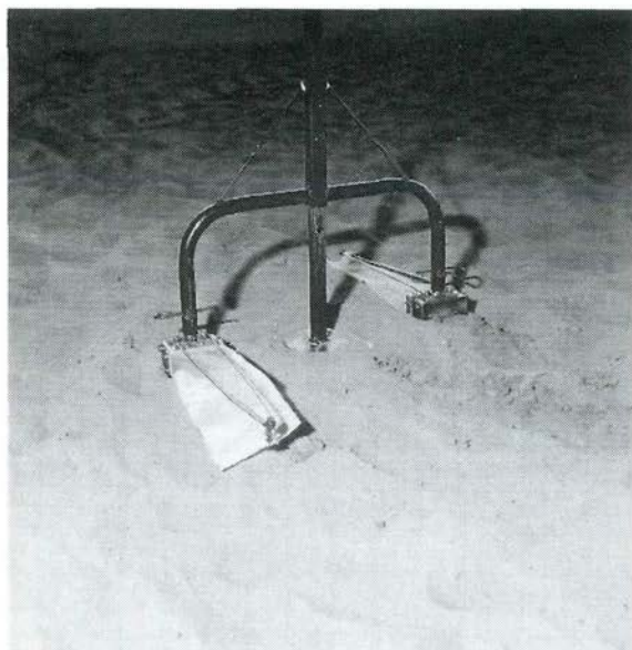
Photo 3.2 Bedload sampler as used in the field.
