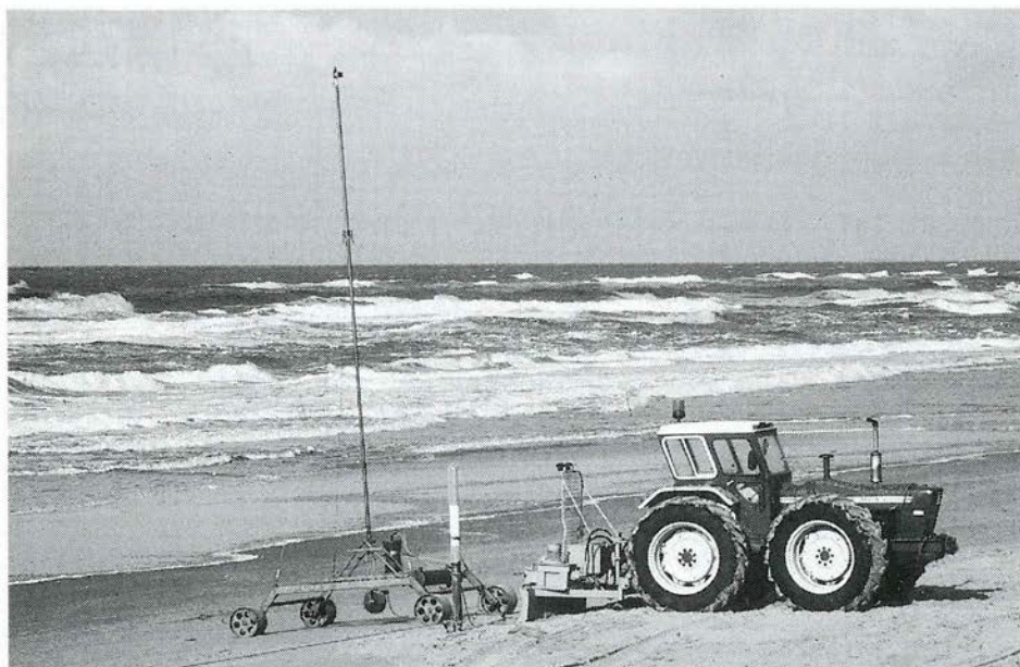
Photo 3.3. Sub-Aquatic Profiler (SAP) positioned in front of Tractor with winch.
