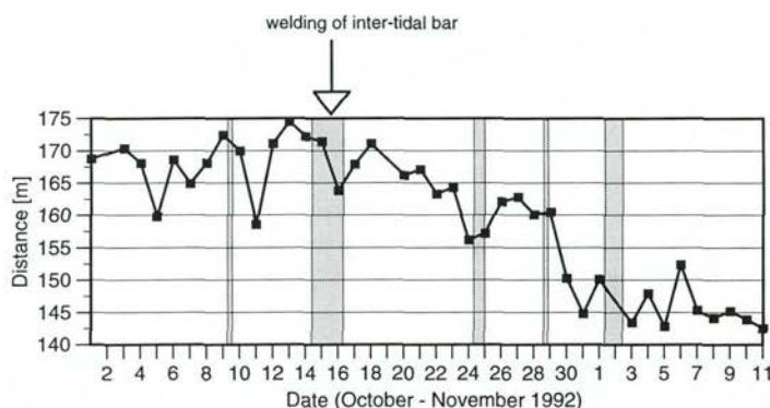
Figure 6.31 The location of the trough of the inner nearshore bar at SAP profile as function of time in 1992. Shaded areas indicate storms.
