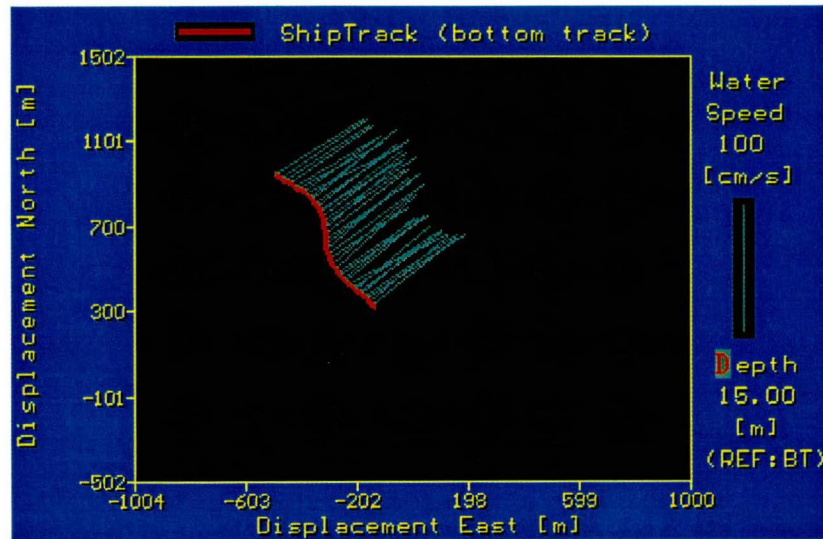
Fig 3.12. Visualization of the shiptrack and velocity vectors measured at 15 m below the water level.
