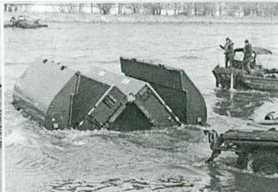
A centre section unfolding in the normal way -- in the background a tugboat waits to capture the unit.
