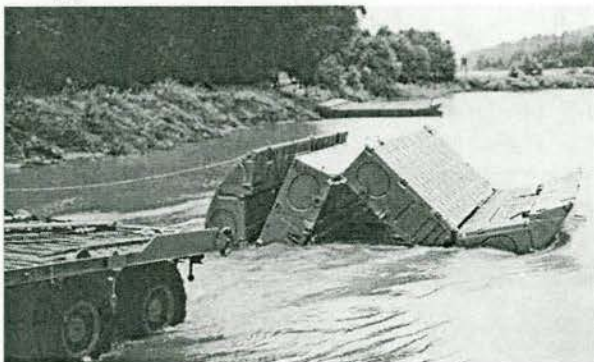
The steel Folding Float Bridge: a centre section unfolds by means of a torsion bar.
