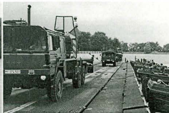
A vehicle drives over the German Army's aluminium Folding Float Bridge.
