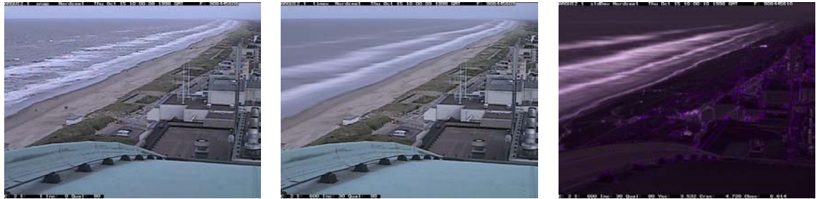
Figure 2.1 Snap shot image (left), Time averaged image (middle) and Variance image
