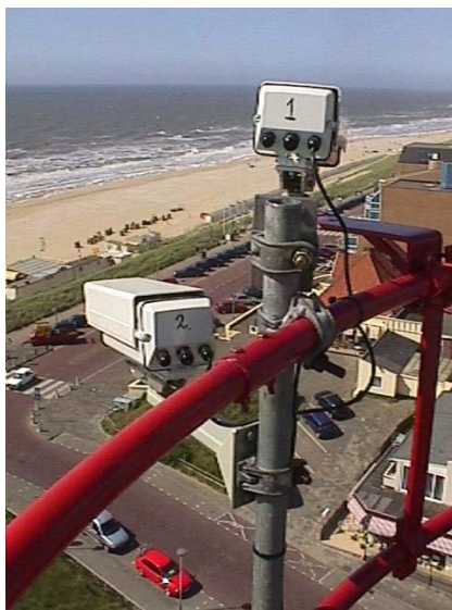
Figure 2.5 Argus cameras on top of the lighthouse 'Jan van Speijk'
