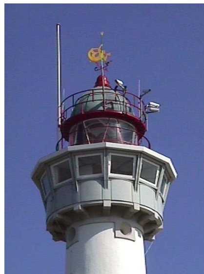
Figure 2.5 Argus cameras on top of the lighthouse 'Jan van Speijk'
