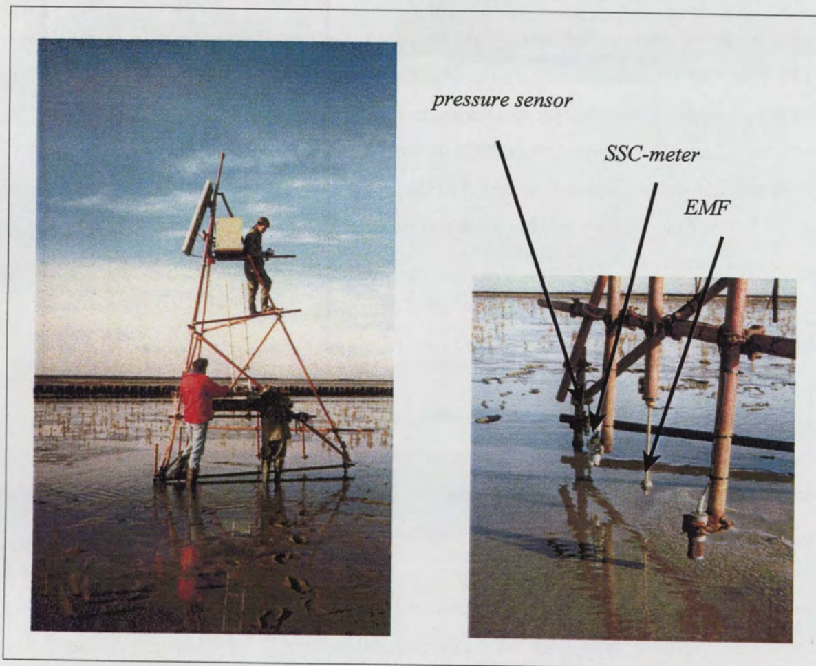
Fig. 4.3: Measuring frame with pressure sensor, electromagnetic flow meter (EMF) and SSC-meter.
