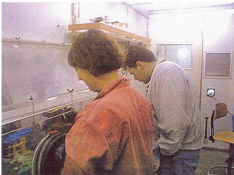
Figure 5 Christelle and Gerard slice a sediment core using the anoxic glove box
