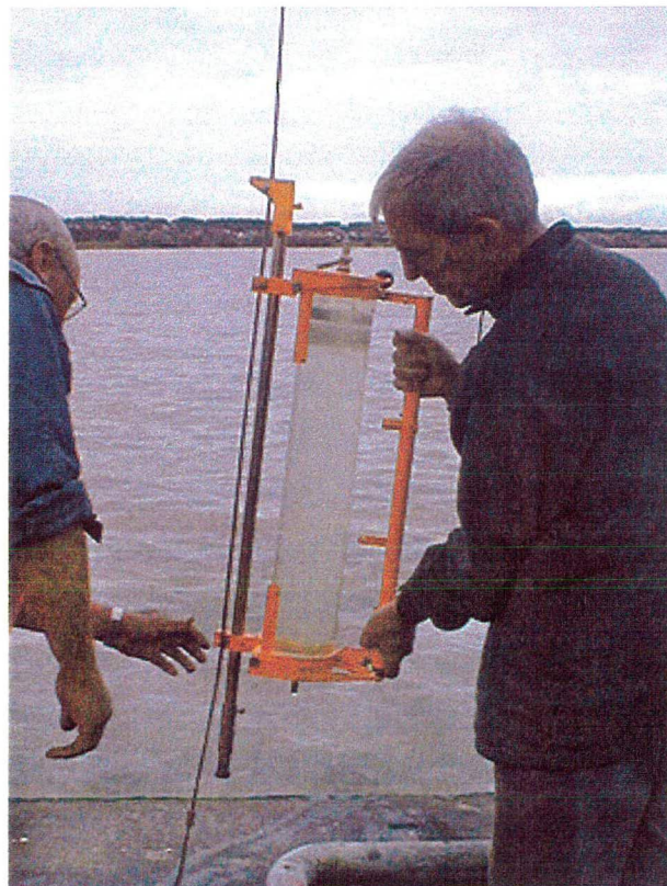
Figure 7 Pieter and Johan prepare the Niskin bottle for bottom water sampling
