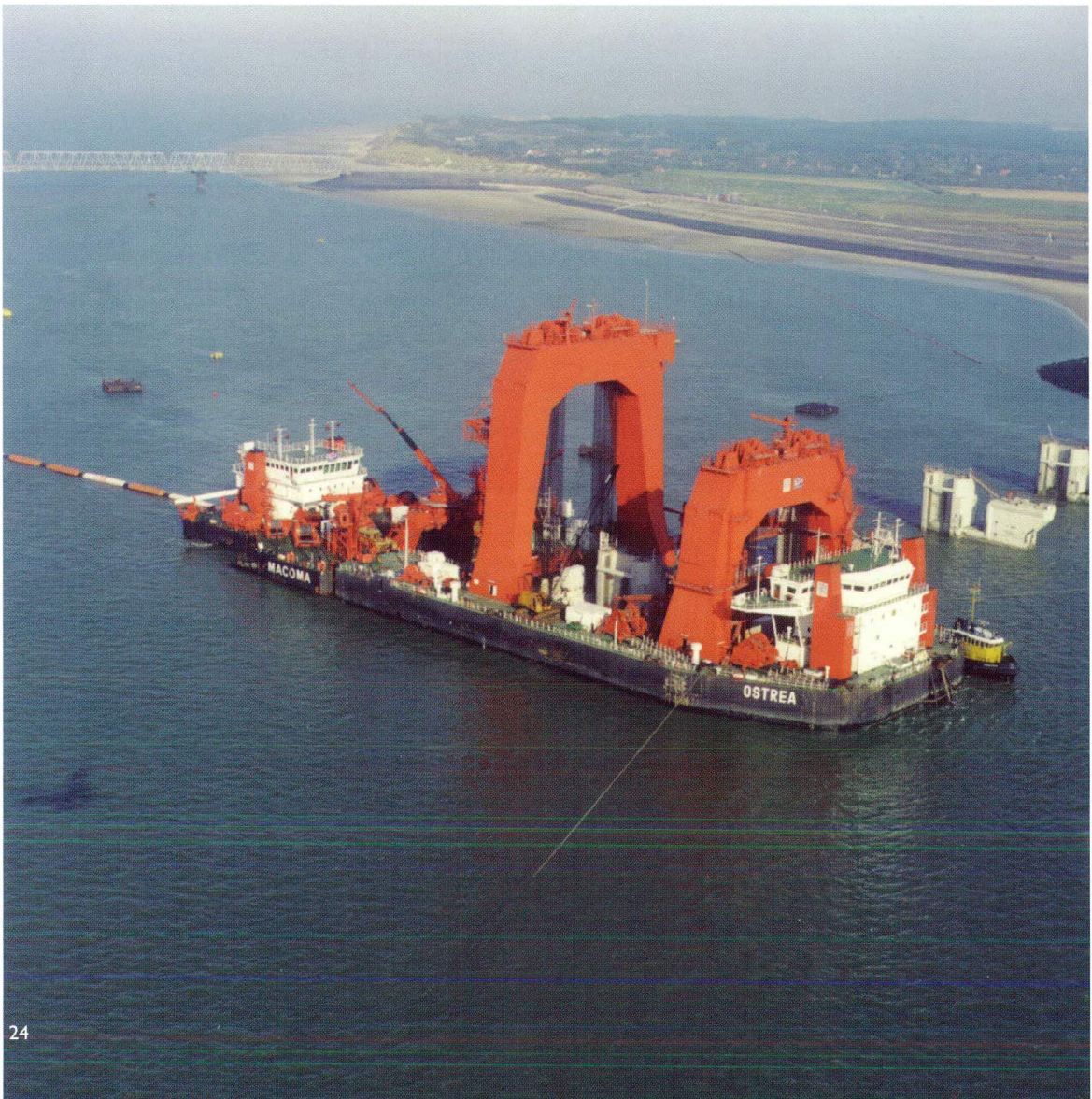
The Ostrea crane vessel and the Macoma mooring and cleansing pontoon shortly after a pier has been installed.
