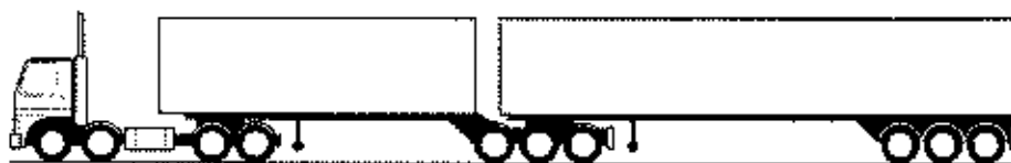
Figure 3 - B Double up to 27.5m long (GVM to 76.5t with container concession)
