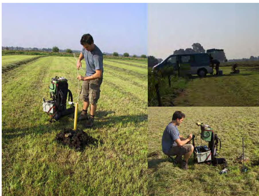
Figure 10 Sampling the upper metre of groundwater (left) and field analysis (down right) on a farm in the sand region.
